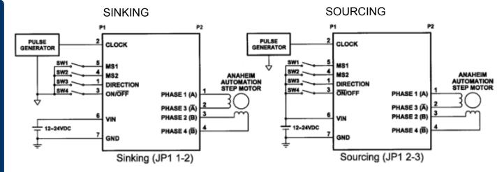
3.5-24 VDC Power Requirements: 12 - 24 VDC Input Signal Voltage Output Current Range: 0.5 - 2.5 Amps (Peak) Storage Temperature: 0°-50° C 200, 400, 800 and 1600 Absolute Maximum 70°C Microstepping Resolution: Steps/Revolution **Driver Temperature** Bipolar, Compatible with 4, 6, and 8 Lead Input Clock Frequency: 0 - 500 KHz **Driver Type** Motors. Series or Parallel Connection
